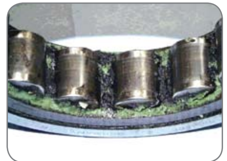
Lubricant degradation caused by electrical discharge currents
