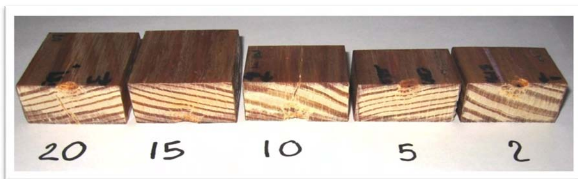
Figure 5-19. Image of samples used on the step-impregnation analysis. Larger impregnation depths may be seen for the longer times.
