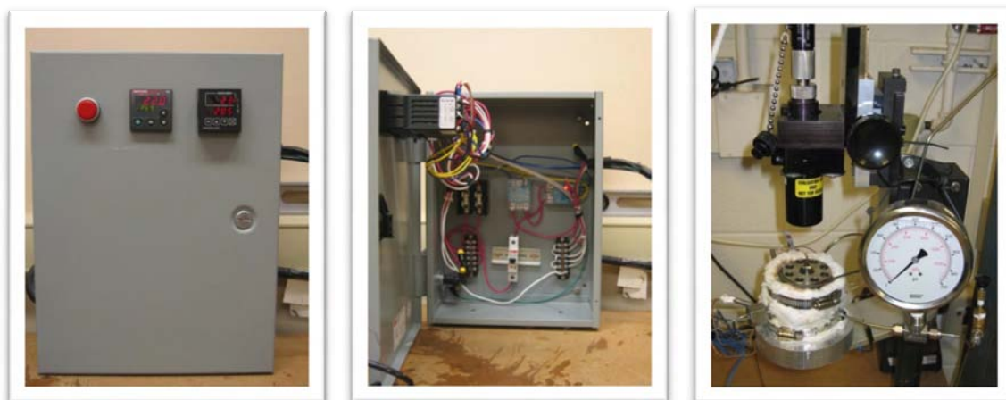
Figure 3-10. Control box (left). Inner control box wiring set-up (middle). Microscope stand mounted reaction chamber (right).
