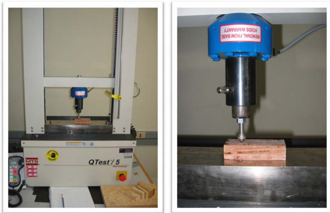
Figure 5-20. Modified MTS tensile/compression tester used for Janka hardness testing of impregnated and unimpregnated wood specimens.
