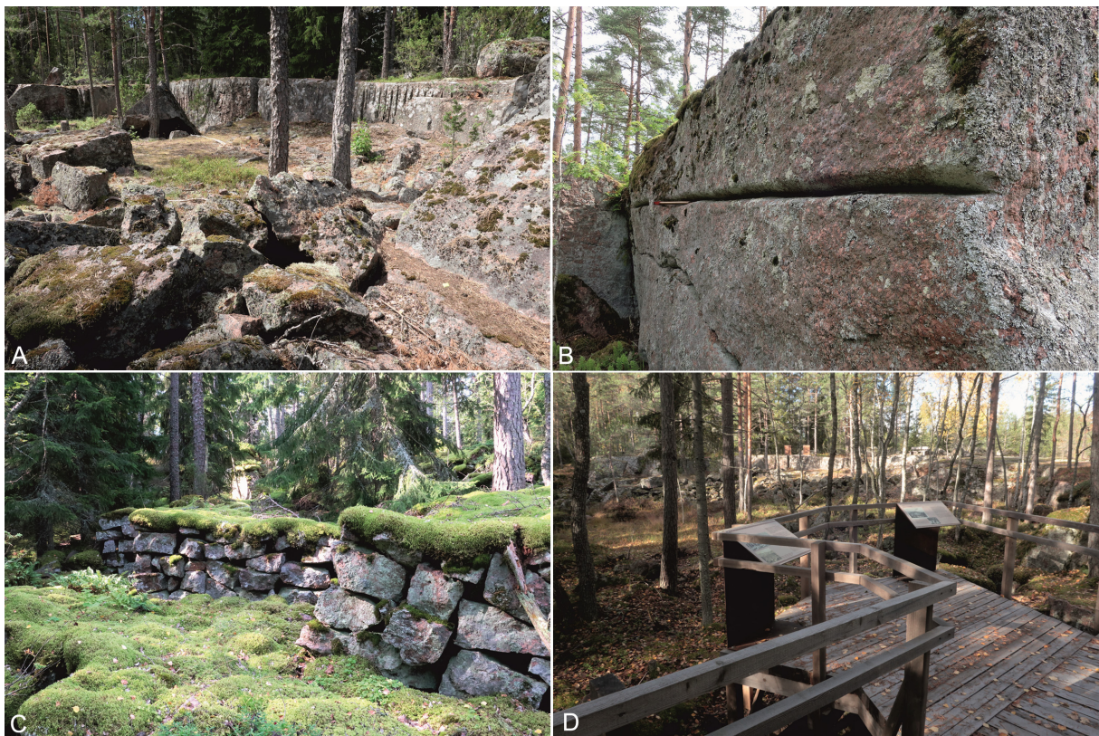
Figure 7. A The historical Hevonniemi quarry for Virolahti pyterlite, from which the famous column of Alexander I was extracted from. Photo: Paavo Härmä. B A subhorizontal V-shaped groove carved in Virolahti pyterlite. Photo: Paavo Härmä. C Semifinished blocks of Virolahti pyterlite stacked in piles in a historical quarry on the island of Korpisaari. Photo: Paavo Härmä. D A tourist route with information signs has been constructed through the area of the Hevonniemi historical quarry. Photo: Paavo Härmä.
