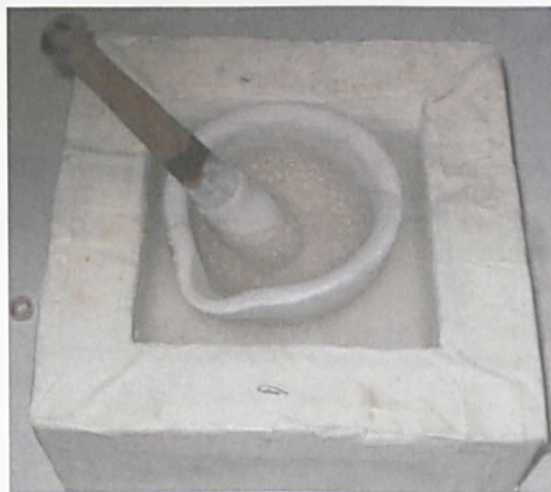
Figure 2.2. Pestle and mortar partially submerged in liquid nitrogen. The sample was ground in the mortar whilst fully submerged in liquid nitrogen.
