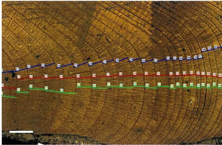
Figure 2 – 9: A section of a digital photo-mosaic (position indicated by the black box in figure 2 – 8). Three series of growth measurements have been taken from this image, (blue, red and green lines). These series were then used to compile an average growth series for the specimen and it is this average growth series which was used in the SHELLCORR analyses. Scale bar = 200um.
