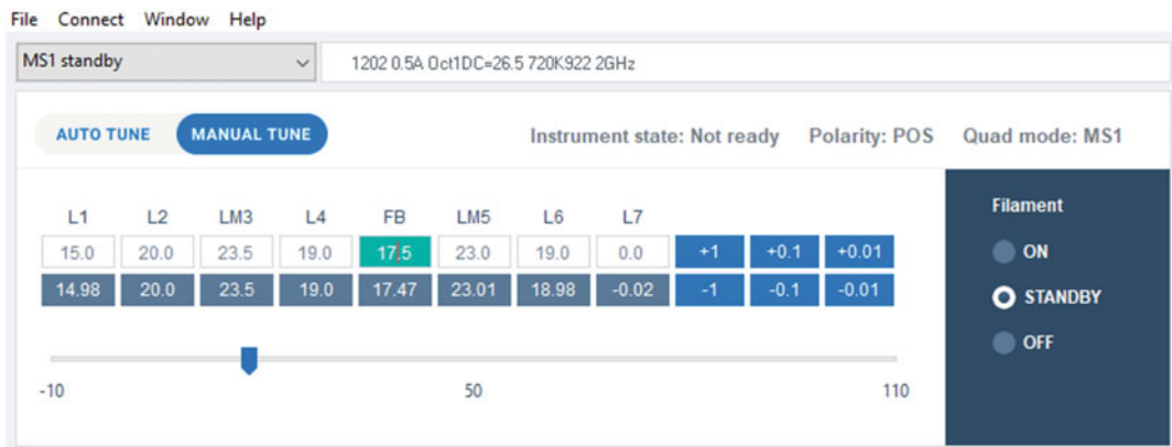
Fig. 3 Tune window for ExD cell controller. ECD profiles are optimized through systematic increases and decreases in lens voltages implemented through +/– controls on the left side of the window
