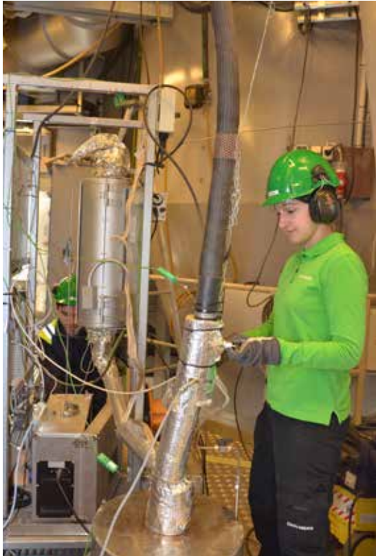
Left: Isabel Cañete Vela introducing gas into the high temperature oven. Right: Teresa Berdugo Vilches in the front and Huong Nguyen in the back preparing an experiment in the external reactor that are fed with gas from the gasifier to allow dedicated investigations to give a more detailed understanding of the process.
