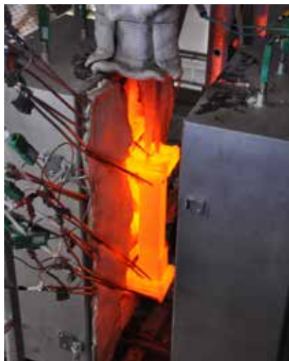
The chemical looping reforming reactor connected to the Chalmers gasifier as part of Fredrik Lind's PhD project. Photo: Henrik Thunman.
