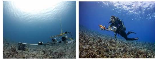
Figure 3: Stereo-BRUVs set-up (left) and Stereo-DOVs transect being completed (right).
