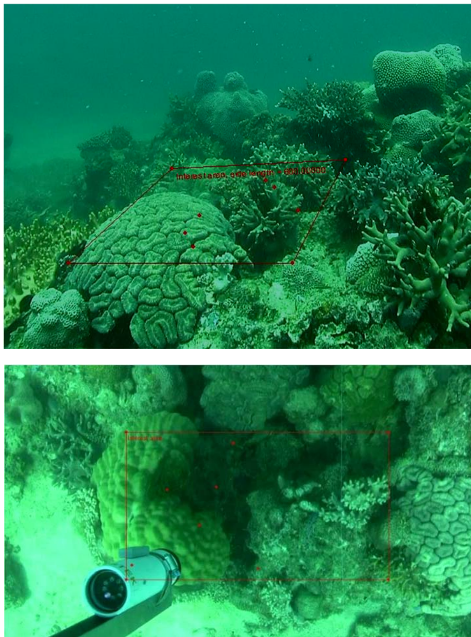
Figure 11.2.1 Calibrated projective transformation (virtual quadrat) projected onto the frame of the (a) forward-DOV and (b) downward-DOV, with six randomly placed points superimposed for benthic identification. The white line seen in image (b) is the biodegradable cotton string. Red text state the 'Interest area, side length=6000.000'.
