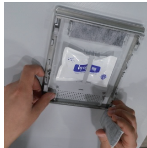
⑤ Open the Hook and insert a new deodorant
