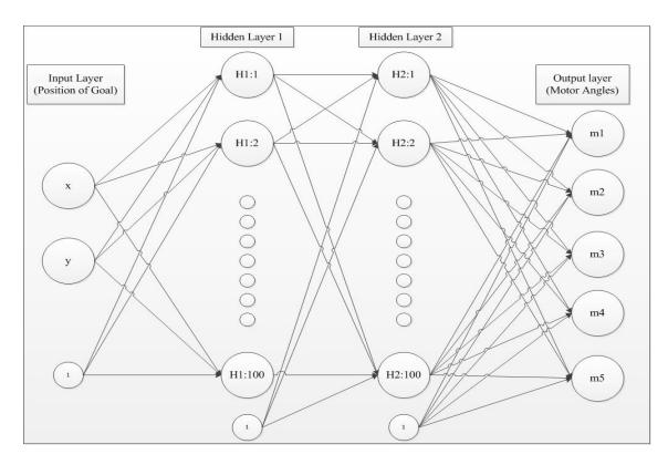
Figure A.2: Artificial Neural Network Architecture
