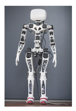
Figure 2.3: Poppy<sup>4</sup>, open source, 3D printed robot
