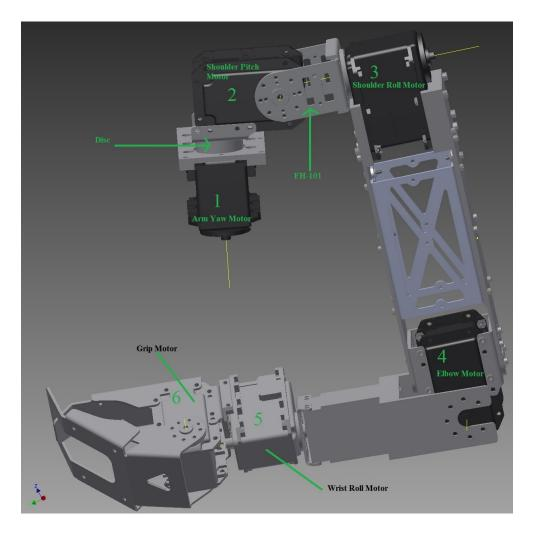
Figure 3.2: New Design of the arm (Left arm). The thin yellow lines show the axis of rotations of their respective motor
