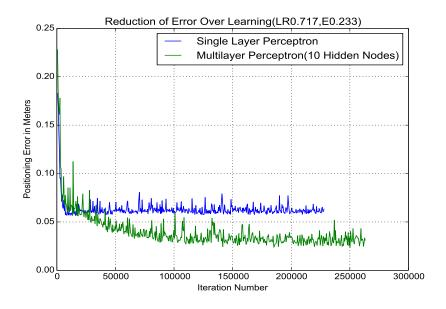
Figure 4.12: Reduction of error over iterations. Positioning error here is the average over the complete testing set
