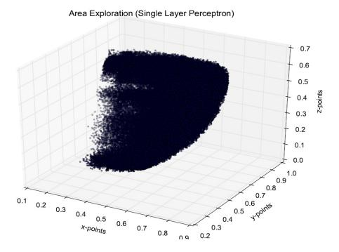
Figure 4.10: Area Explored by the SLP (LR0.717, E0.233 & 0 Hidden Nodes). The robot origion is at (x,y,z = 0.56, 0.35, 0.31)
