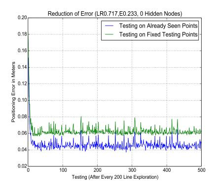
Figure 4.9: Average Testing Error over Seen and Fixed Testing sets For Single Layer Perceptron
