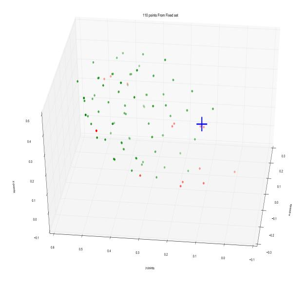
Figure C.1: Fixed points testing points-red shows the points with absolute error more than 4cm and green show less than 4cm. Blue cross show the center of the robot model (LR0.717, E0.233 & 10 Hidden Nodes)
