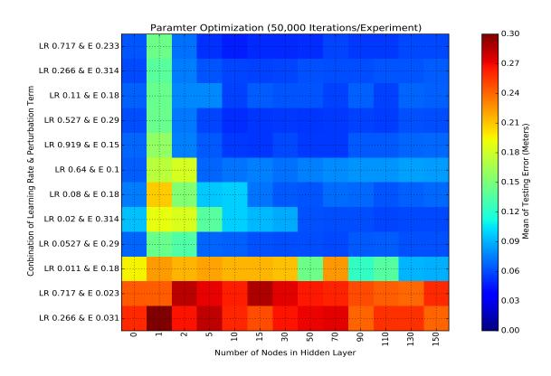
Figure 4.3: The plot shows the result of parameter exploration for higher learning rate and higher perturbation values than 4.2. The heat values in the map are the mean of average positioning error over testing cycles.
