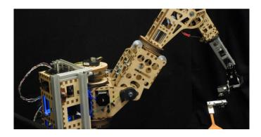
Figure 2.1: A low cost Robot Manupulator with 7 DOF
