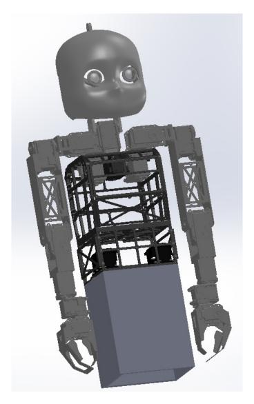
Figure 3.8: Nicu Torso Assembly - Solid Works
