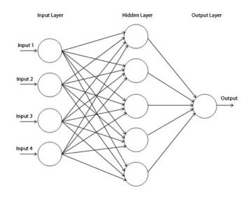
Figure 1.5: Model of Multi Layer Perceptron
