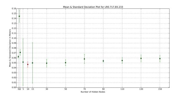
Figure 4.4: Mean & Standard Deviation of average positioning error (over testing cycles for best case of LR0.717 & E0.233). For optimal number of nodes the best result (against 10 Hidden Nodes) obtained can be viewed in red color. These experiments shows the exploration results for 50,000 iteration each.
