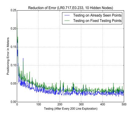
Figure 4.6: Average testing Error over Seen and Fixed Testing Sets
