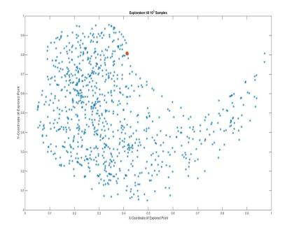
Figure A.5: Workspace exploration till  $10^3$  samples. Red dot in the figure shows the origin of the arm.
