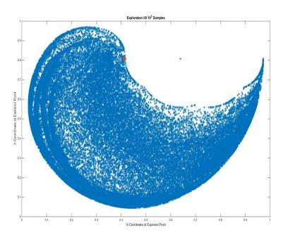
Figure A.7: Workspace exploration till  $10^5$  samples. Red dot in the figure shows the origin of the arm.
