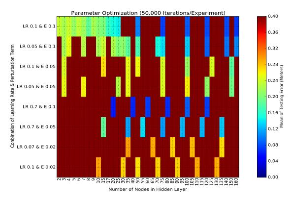
Figure 4.2: The plot shows the result of random parameter exploration. The maximum mean error is about 0.3 meters. The heat values in the map corresponds to the mean of average positioning error over the testing cycles. The dark red part shows the region for which the experiments were not performed
