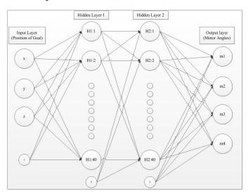
Figure 5.3: Artificial Neural Network Architecture for SURALP
