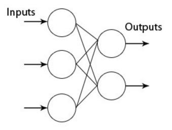
Figure 1.4: Model of Single Layer Perceptron
