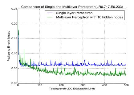
Figure 4.11: Comparison of fixed testing points error of MLP & SLP. Positioning error here is the average over the complete test set.
