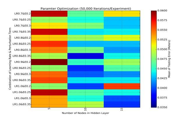
Figure 4.5: The plot shows the result of parameter exploration for parameters close to the best case (LR0.717 & E0.233 & 10 Hidden Nodes). The heat values in the map are the mean of positioning error over testing cycles.
