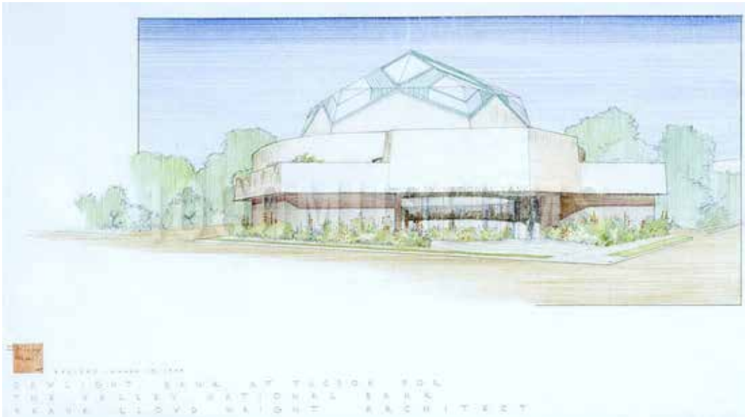
FIG. 5.23 Example of Wright's use of the polyhedron: Vallet National Bank, Tucson (AZ), 1949. Courtesy of FLLWFA (MOMA / AA&FALCU)]
