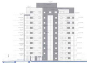
FIG. 5.63 Section of a constructed building. 2008. (Drom HaSharon Committee). Note the upper floors are larger than the lower ones
