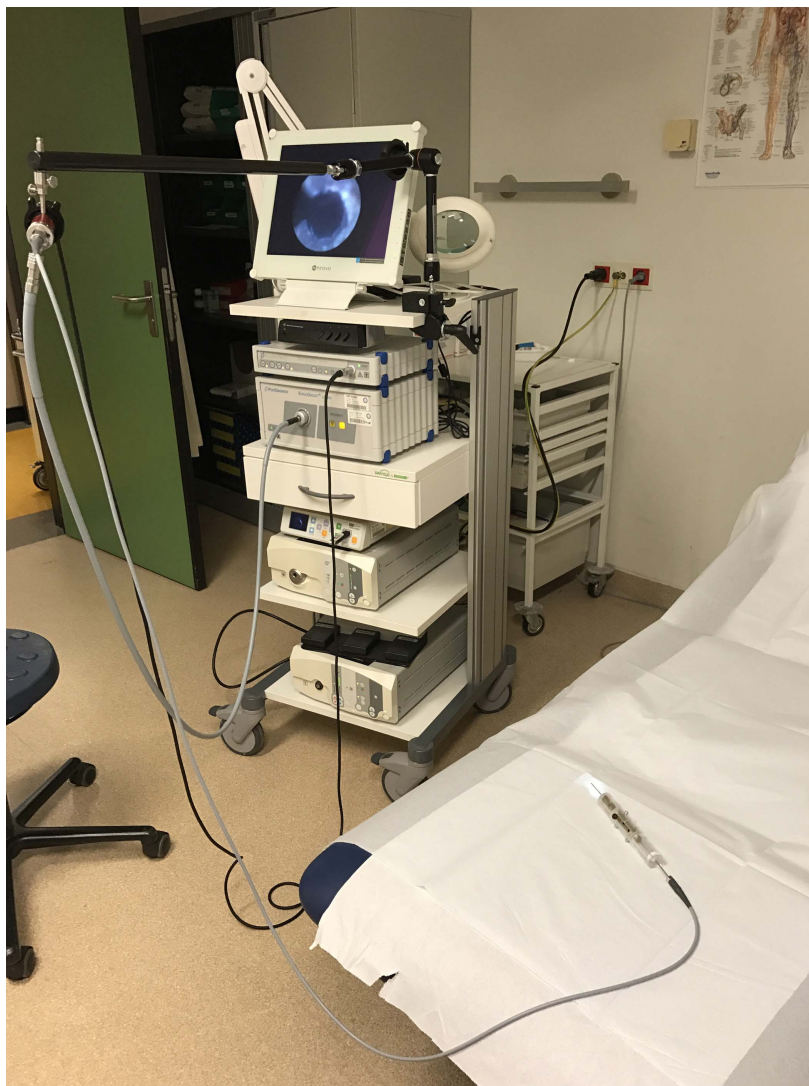
Figure 15. Clinical Experimental Facility at University Medical Center (Utrecht, the Netherlands). The experimental facility consisted of the biopsy needle integrated with the micro-endoscope connected to the imaging equipment.
