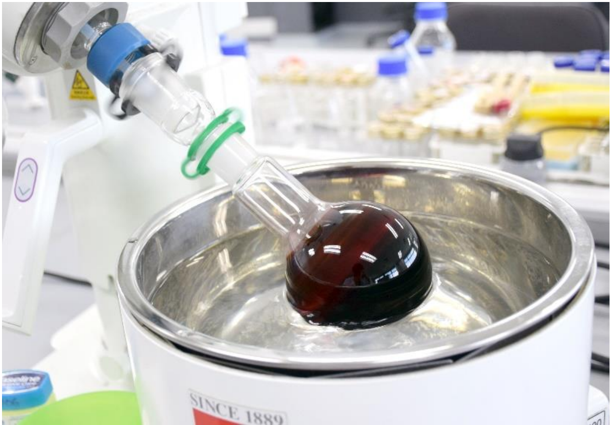
Figure 2.9 The methanolic leaf extracts of N. rafflesiana in a rotary evaporator. Note the red color of the extracts.
