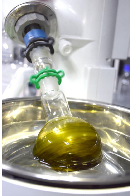
Figure 2.8 The methanolic leaf extracts of N. ampullaria in a rotary evaporator. Note the green color of the extracts.
