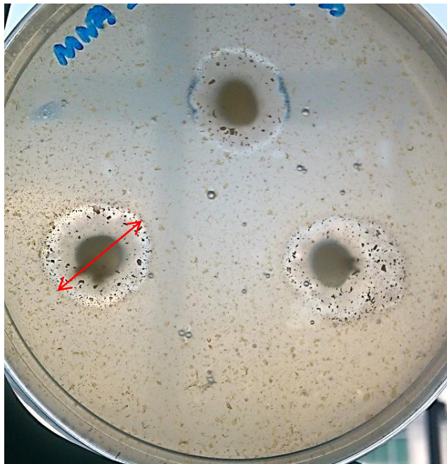
Figure 8 PUR clearance zone indicated by a change from opaque to transparent medium.
