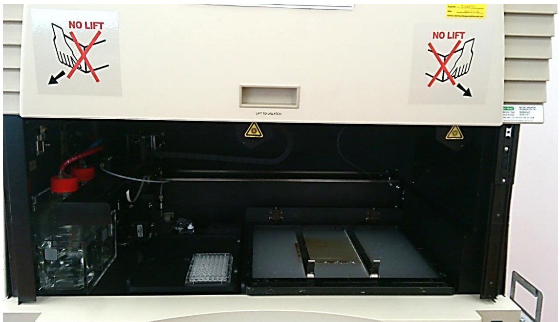
Figure 18 Spot Cutter System used to excise protein spots of significance change in the abundance.
