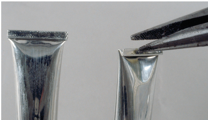
Fig. 5. Crimping ends of tubes with pliers
