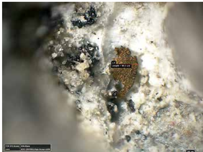
FIG. 7. Detail of fig. 3, showing a fragment of gold leaf in the pupil's cavity (right eye). 3D Digital Microscopy, X 500. The fact that this fragment (ca. 80 x 120 µm) is partially trapped in white concretions confirms that it is an ancient pollution
