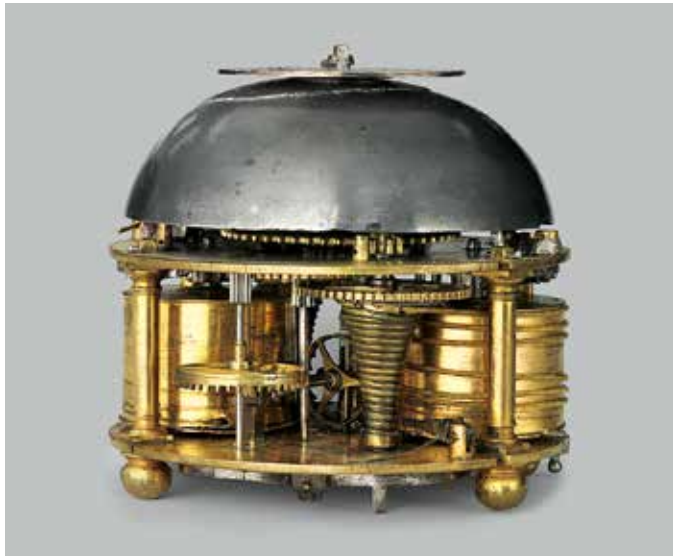
The movement with the bell and dial
