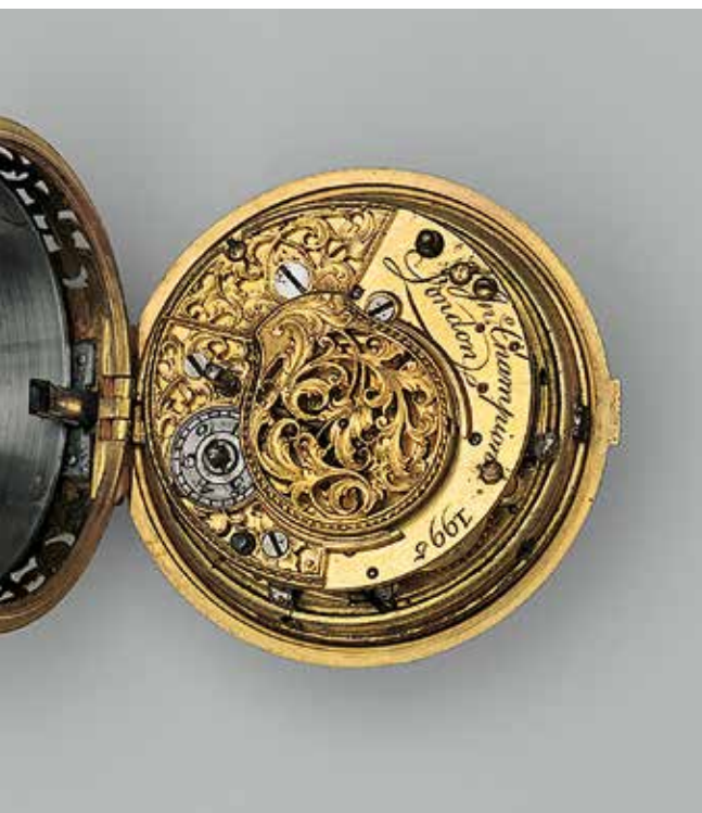
The inner case open to show the back plate of the Champion watch
