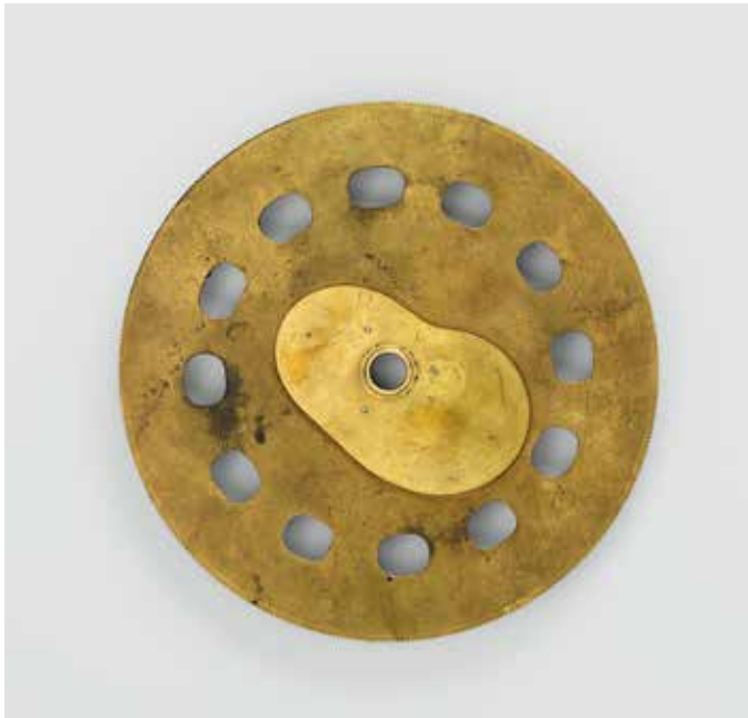
The reverse side of the calendar plate with the kidney-shaped element, allowing the solar hand to register true solar time
