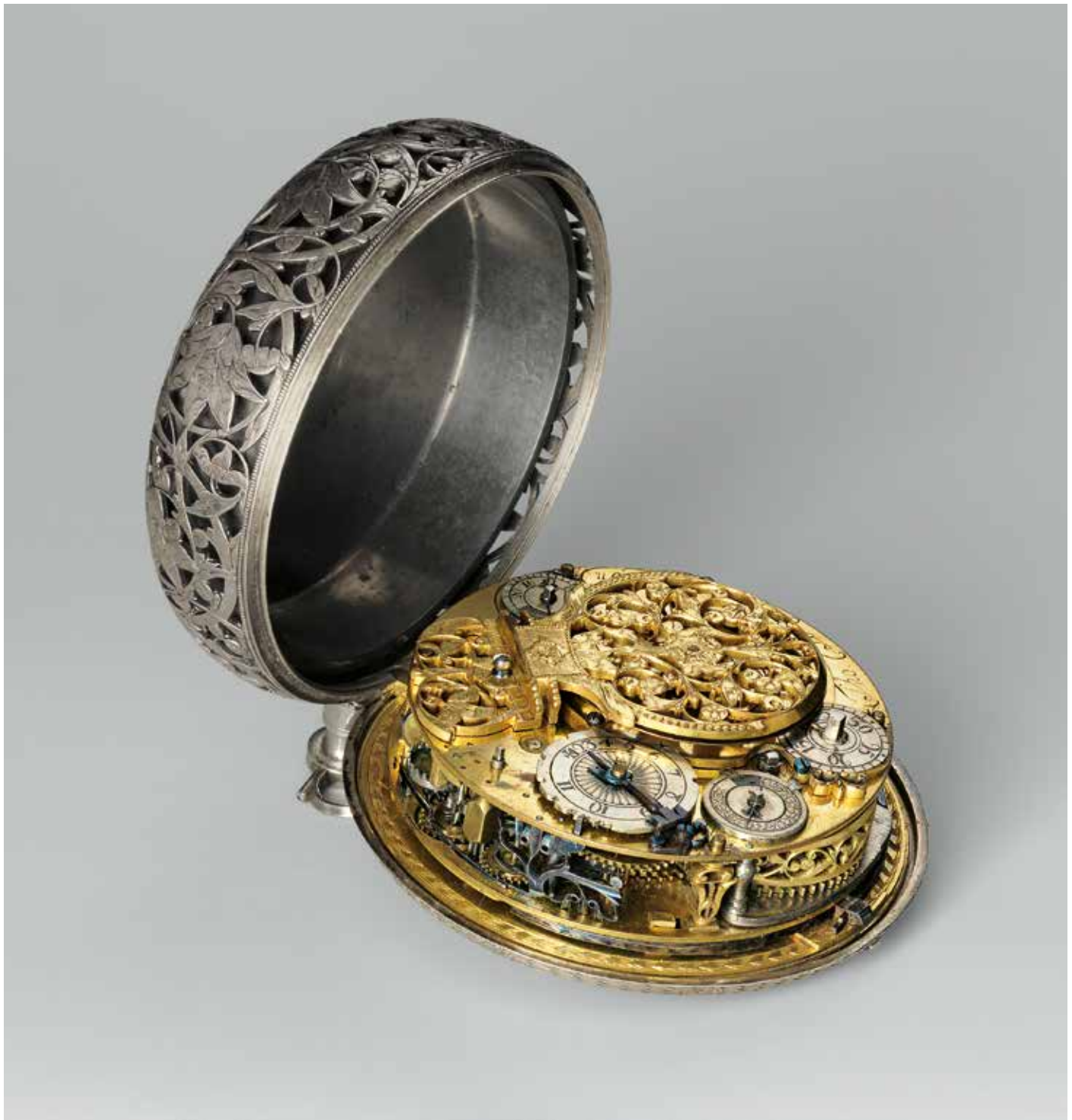
The watchcase open to show the movement
