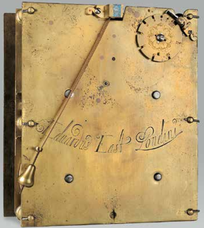
Back plate of the movement with a short pendulum, count wheel, and the signature of the clockmaker
