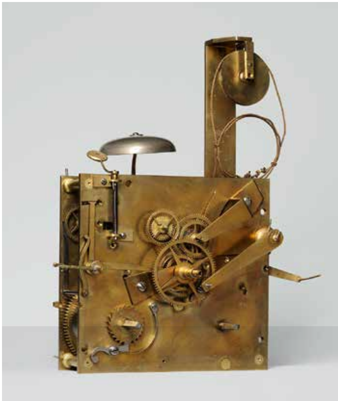
The view of the movement, showing the front plate with the epicyclic system for the display of both the true solar time and mean time
