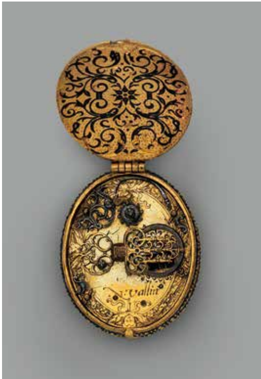
The back cover of the case open to display the back plate of the movement and the signature of the watchmaker
