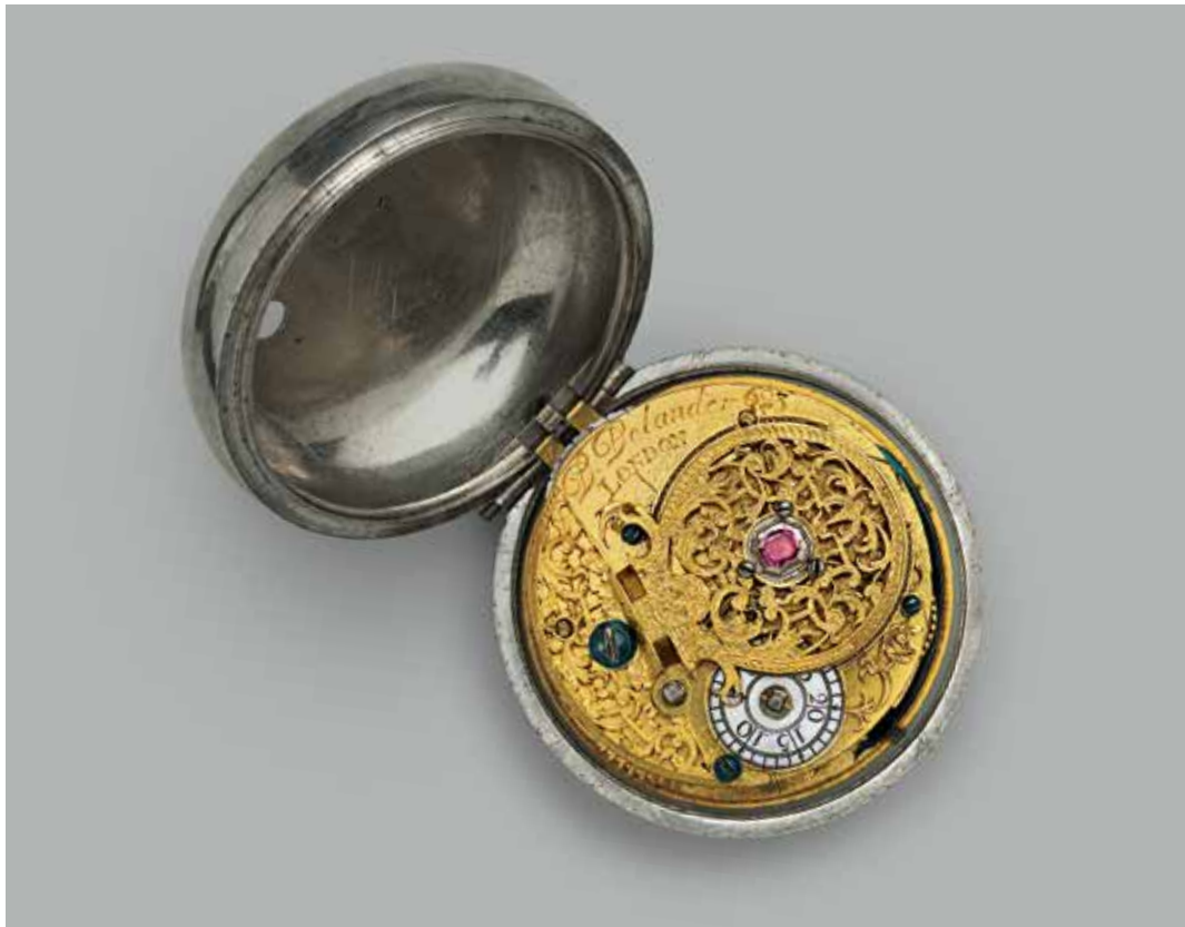
top: Detail of the table of the balance cock with the half-drilled diamond endstone bottom: View of the open watch to show the back plate
