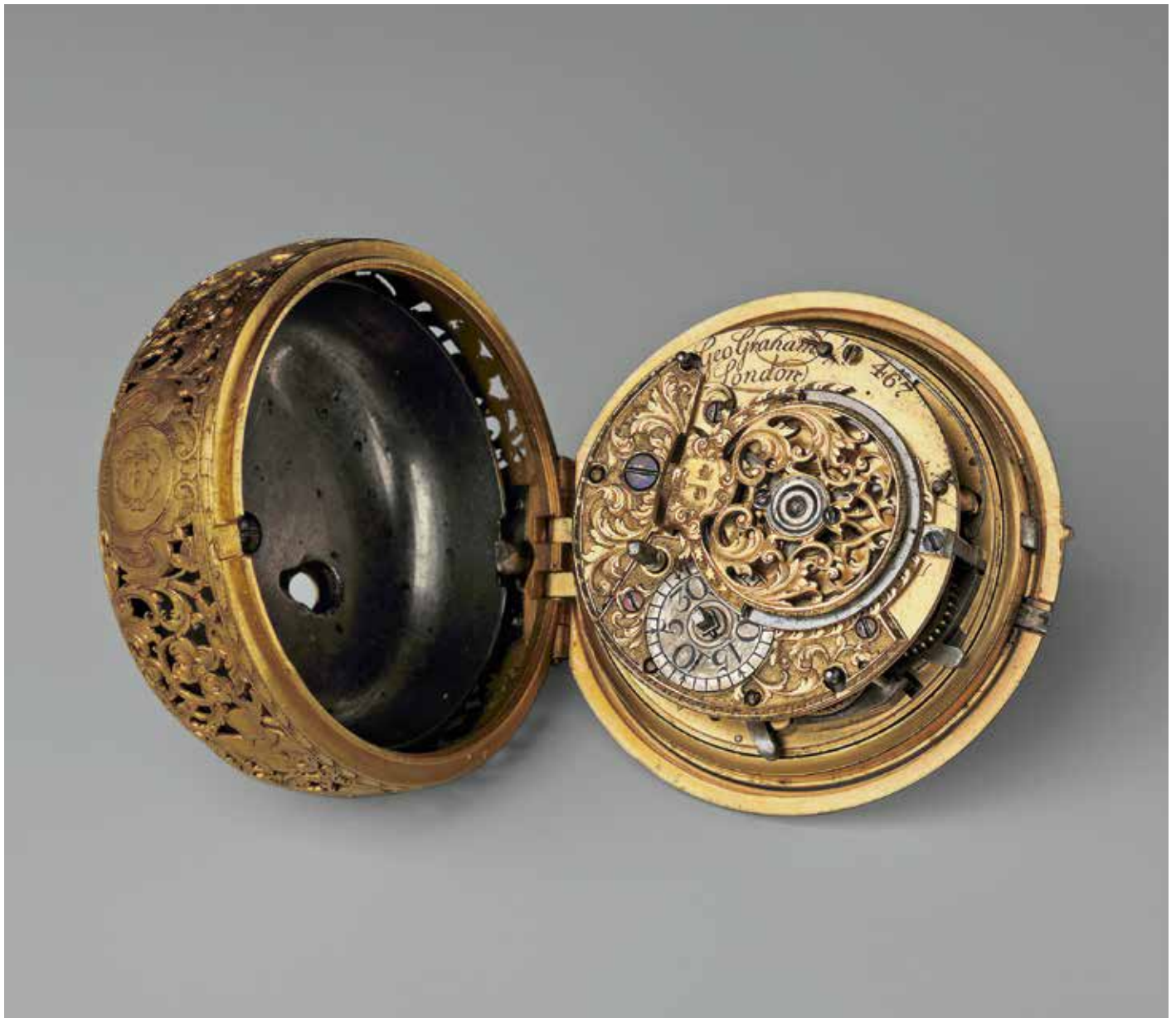
Inner case open to show the back plate of Graham watch
