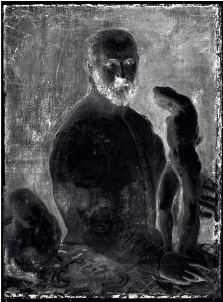
fig. 8 Iron distribution map acquired by XRF imaging of Alessandro Vittoria (fig. 1). Iron is the primary component of earth pigments, such as ochers, sienna, and various brown and red earths, which are used in paint mixtures to deepen tones and model form.
