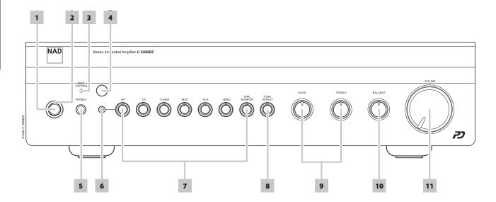
1 STANDBY: With the rear panel POWER switch set to ON position, press this button to switch ON the C 326BEE from standby mode. The Standby LED indicator will turn from amber to blue. Pressing the STANDBY button again turns the unit back to standby mode.
