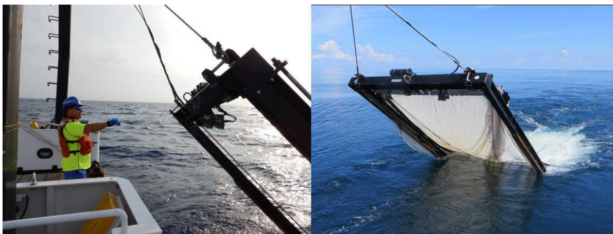
Figure 3 - 10-m 2 MOCNESS (MOC-10) unit being retrieved (left) and deployed (right) on the R/V Point Sur during DEEPEND cruise DP04.
