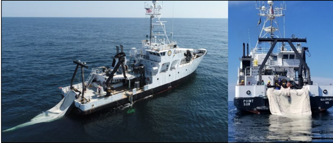
Figure 5. 10-m 2 MOCNESS (MOC-10) unit being retrieved (left) and codends being retrieved (right) on the R/V Point Sur during DEEPEND cruise DP06. Photo: DEEPEND 2018/Danté Fenolio.
