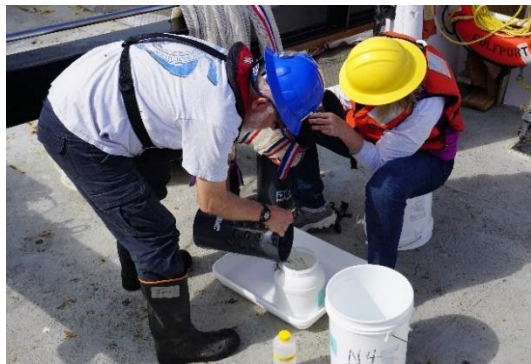
Figure 6. (Left) MOC-10 codend being collected into a cold-water bucket, and (right) depth sampling scheme.
