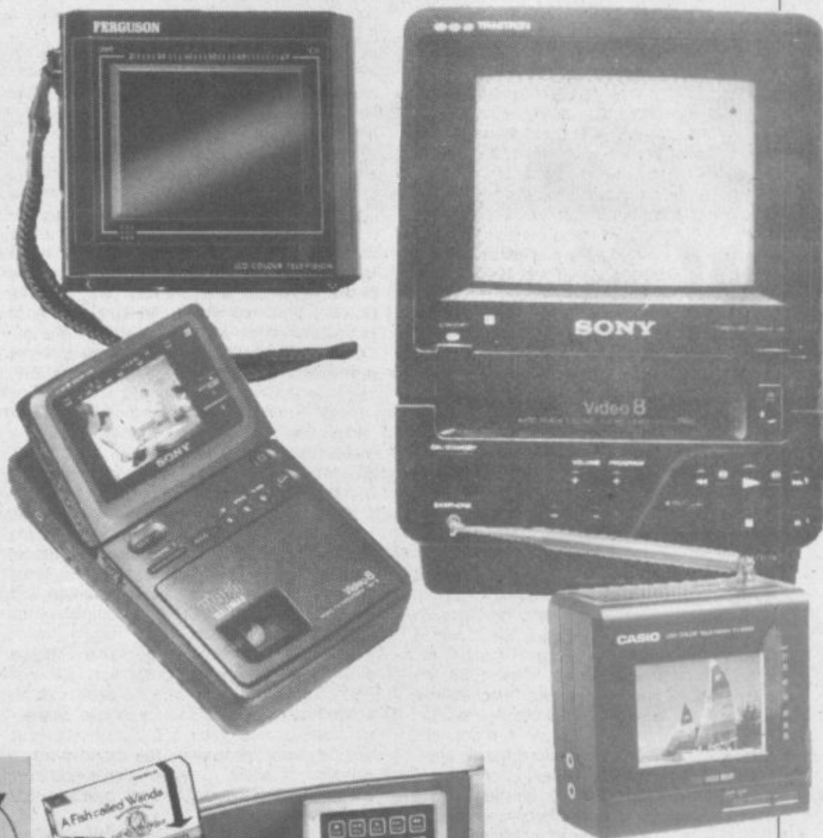
Above, clockwise from the top left: The Ferguson PTV02, with 3-inch LCD screen, the Sony EV-DT1 with 6-inch screen, Casio TV6500 at 2.7 inches, and the amazing Sony GV-8 Video Walkman with a 3-inch screen. The appliances shown are not in scale with each other!
