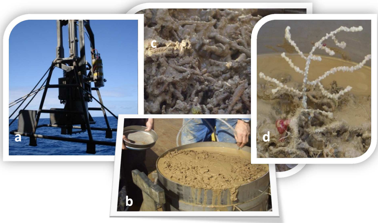
Figure 10. Sampling processing onboard the R. V. Pelagia (cruise 64PE268). a) TV-guided box corer with mounted camera system; b) sediment washing for fauna sampling; c) subsampler of the box-core; d) fragment of coral retrieved by the box corer sampler. © Photos by Clara Rodrigues.
