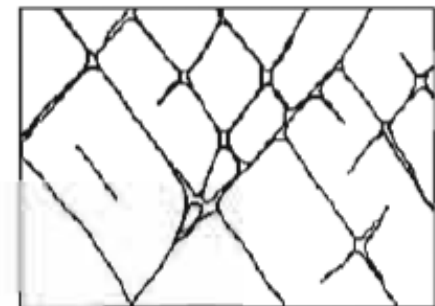
Solid rocks rendered porous by fracturing
