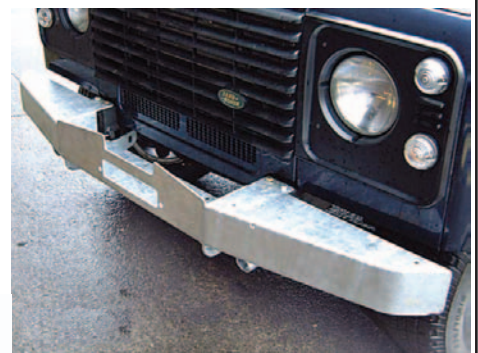
Winch bumper; Front bumper incorporating winch frame. Suitable for the following winches: Warn 6000 & 8000 M & MX series, Warn XD9000, Superwinch X6 CD & X9, T-Max. Incorporates jacking points. Available in black nylon or galvanised finish.
