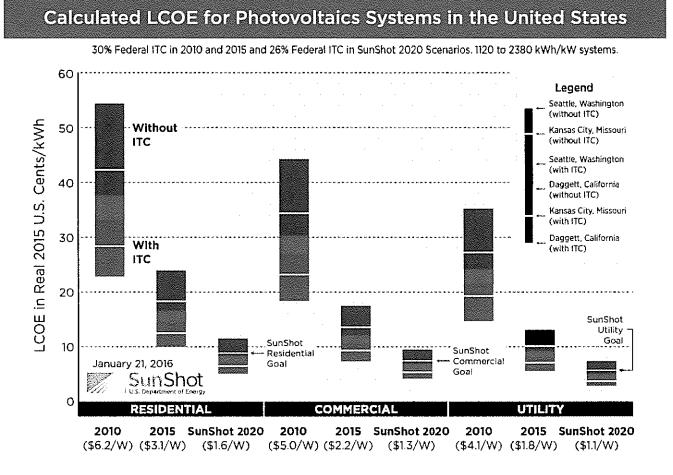
Figure 1. Solar PV LCOE - historical, current, and 2020 targets
