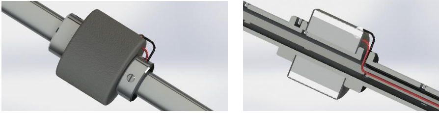
Fig 3.29. Layout of a single transducer introduced in the array bar. On the left image; detail of the transducer holding through screws. The right figure show the detail of the ceramic cable connection and its itinerary through the bar.
