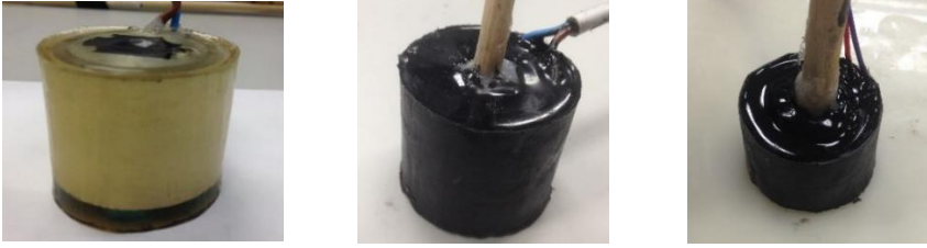
Fig. 3.12. Piezo-ceramic large tube with aluminium backing and RoyaPox 511 moulding (left); Piezo-ceramic large tube with aluminium backing and polyurethane EL241F moulding (middle); Piezo-ceramic small tube with aluminium backing and polyurethane EL241F moulding (right).
