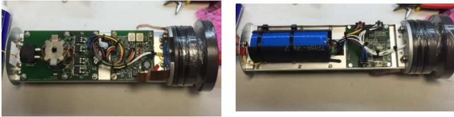
Fig 2.18. Upper and lower views of the AB electronic boards.
