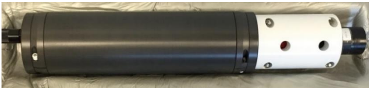
Fig 2.22. Complete Acoustic Beacon
