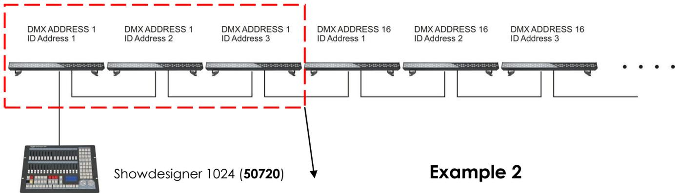
The figure above shows a simple DMX layout. All 3 Spectral CYC2000's have different ID addresses, which allows the user to collectively control a group of 3 Spectral CYC2000's with the same DMX address by setting CH15 to 0, or to control each Spectral CYC2000 independently by first selecting the DMX address and then by using CH15 to locate the target ID address.
