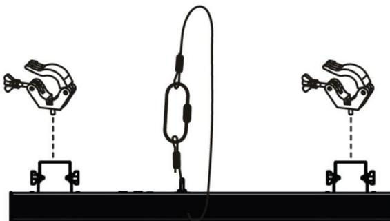
The Spectral CYC2000 can be mounted in a hanging position (Fig. Above) or Upright (Fig. Below), using the support brackets. Mounting the Spectral CYC2000 with a clamp or any other mounting bracket is recommended, depending on the requirements of your application.
