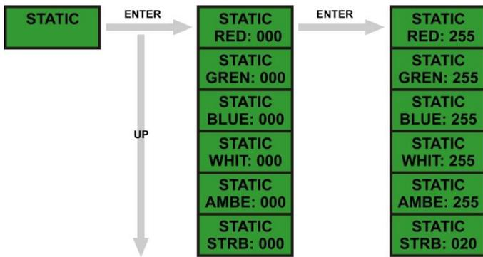
When you press ENTER in menu Static color, you have to use DOWN to scroll through this menu. Use the UP/DOWN buttons to change the static colors (Red, Green, Blue, White, Amber) or the strobe speed (0-20Hz). Press MENU to go 1 step back. You can combine RED, GREEN, BLUE, WHITE and AMBER to create an infinite range of colors (0-255).
