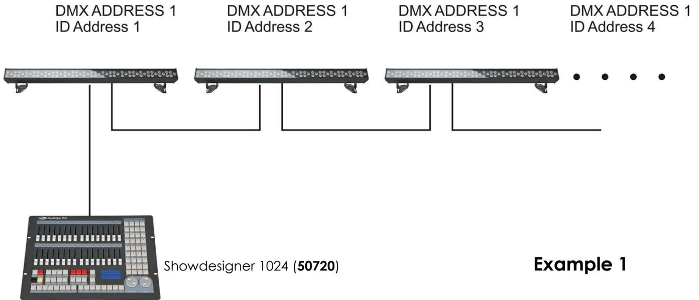
The figure above shows a simple DMX layout. All the Spectral CYC2000's have different ID addresses which allows the user to collectively control the whole group of Spectral CYC2000's with the same DMX address by setting CH15 to 0, or to control each Spectral CYC2000 independently by first selecting the DMX address and then by using CH15 to locate the target ID address.
