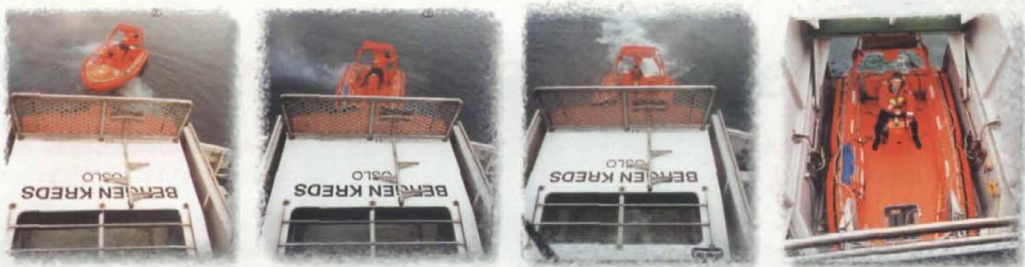
Above: Launching and recovering the daughter boat is rapid and simple.
