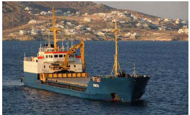
Breadbox Acacia 8843862. An ex GDR Navy tug, she was lengthened from 76 to 90 m and became a general cargo carrier.
