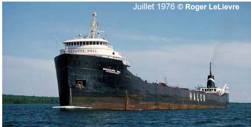
Canadian Miner (ex-Lemoyne (2), ex-Maplecliffe Hall). Foreword section built in 1965 at Lauzon by George T. Davie & Sons Ltd, stern section at Montreal by Canadian Vickers Shipyard Ltd and assembled at Lauzon.
