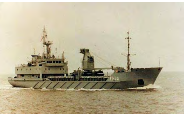
Breadbox Acacia 8843862. An ex GDR Navy tug, she was lengthened from 76 to 90 m and became a general cargo carrier.
