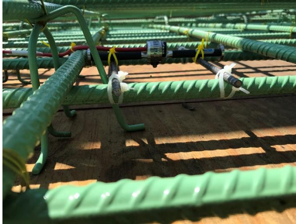
Figure 32. Embedded strain gage placement
