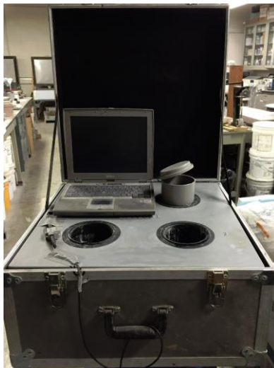
Figure 14. Calorimetry test device for measuring the temperature development of concrete
