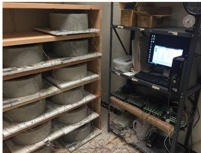
Figure 16. Restrained shrinkage ring test apparatus
