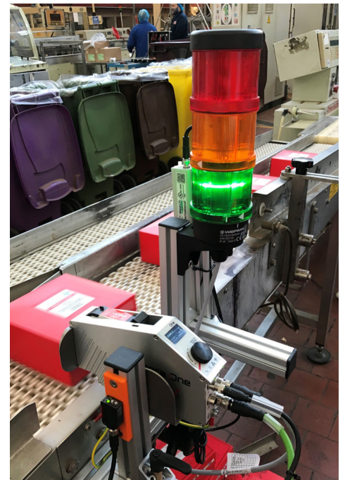
Integra with beacon on conveyor
