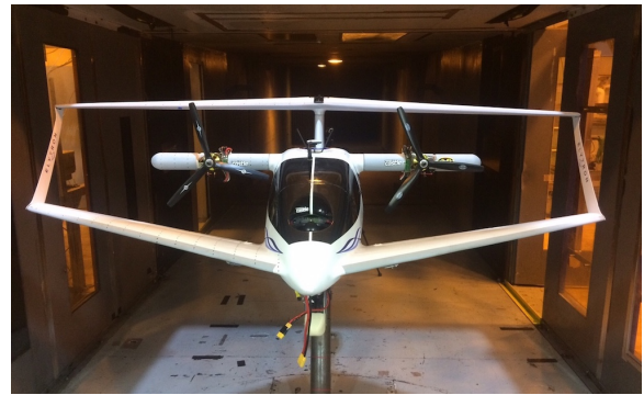
Fig. 1. Elytron 4S UAV in the US Army 7x10 subsonic wind tunnel at NASA Ames Research Center.
