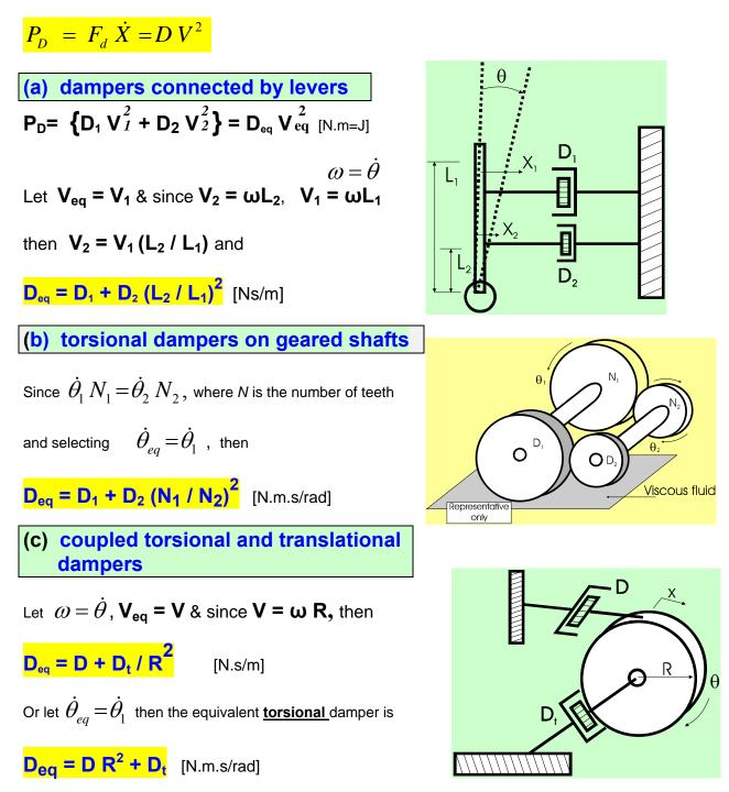
**Note:** in (a) thru (c) one of the dashpot ends is connected to ground.
