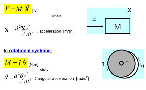
With  $\int [N.m.s^2/rad=kg.m^2]$  as the mass moment of inertia.
