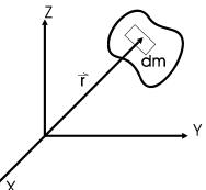
where  $\rho$ : mass density, **V**: body volume, **r**: distance from reference axis to **dm** =  $\rho$  **dV**
