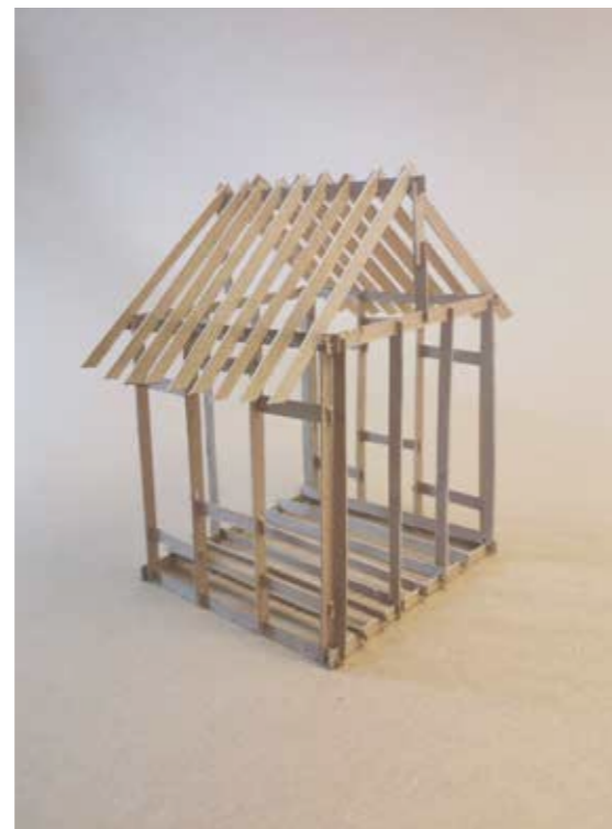
3D sketching exploring the assembly of a timber frame piece by piece
