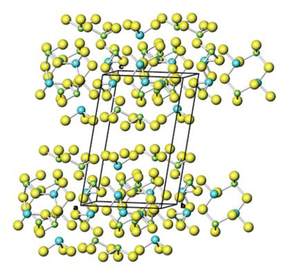
FIG. 8. The distribution of short As(Sb)–S bonds in the structure of gabrielite. S atoms are yellow, As, yellow-green (smaller), and mixed As–Sb positions, turquoise (larger).
