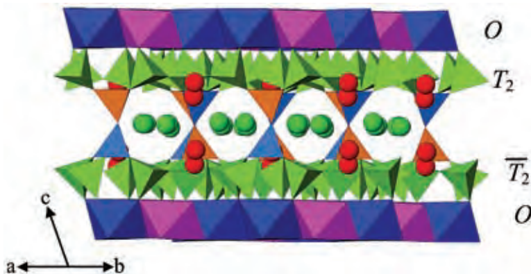
FIG. 3. The OT_2\bar{T}_2O module in lalondeite. The six-membered silicate rings (light green tetrahedra) are cross-linked by Si_3O_4 (orange) and Si_6O_4 (blue) tetrahedra. The closest-packed O layer is composed of NaO_6 (purple) and CaO_6 (blue) octahedra. The H_2O molecules are shown as green spheres, and the disordered Na_{2a,b} ions, as red spheres.
