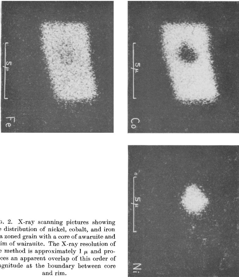
FIG. 2. X-ray scanning pictures showing the distribution of nickel, cobalt, and iron in a zoned grain with a core of awaruite and a rim of wairauite. The X-ray resolution of the method is approximately  $1 \mu$  and produces an apparent overlap of this order of magnitude at the boundary between core and rim.
