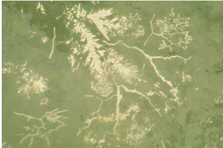
FIG. 14. Photomicrograph of a polished section in vertical illumination, showing veinlets and fern-like fronds of the alteration product of oosterboschite (white) in a matrix of malachite (light grey) and quartz (dark grey). Width of field is 0.2 mm.
