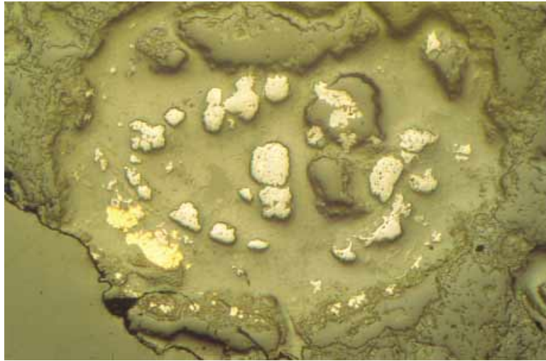
FIG. 5. Photomicrograph of polished section in vertical illumination showing a nodule of mineralized malachite containing grains of Pd oxides (grey under the microscope but pale yellow in this photo) and gold (bright yellow); the darker high-relief grains are quartz. Width of field is 2.2 mm.
