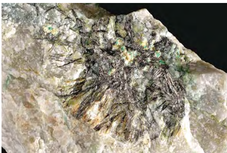
FIG. 2. Pizgrischite crystals spray partially altered into malachite (green) and bismutite (yellow) in a fine-grained quartz matrix. Horizontal field of view is 5 cm. Holotype sample MGL #58622. Photo and courtesy S. Ansermet.
