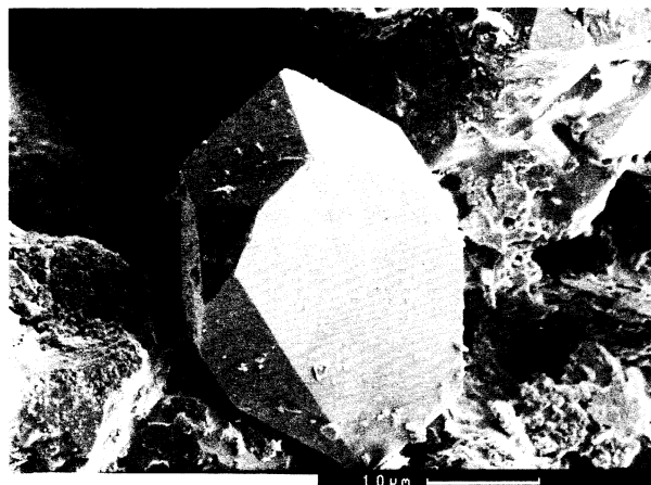
Fig. 1. SEM photograph of a synthetic ammonium feldspar crystal grown at 600 °C and 2 kbar. Flaky material on both sides of the crystal is carbon substrate material.
