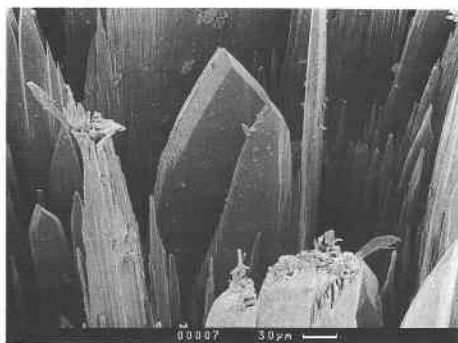
Fig. 1. SEM image of nchwaningite crystals.
