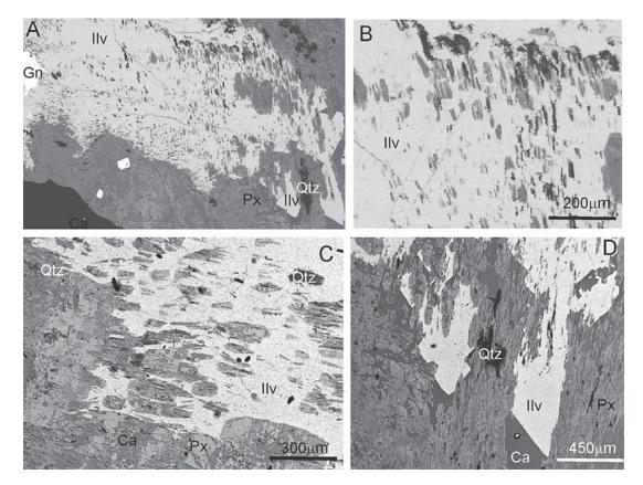
FIG. 10. BSE images of manganilvaite replacing radiating aggregate of pyroxene crystals. We present a general view (A) and details from its upper (B) and lower (C and D) parts. The numerous, partly carbonatized relics of pyroxene preserve their original radiating, slightly fan-like orientation.
