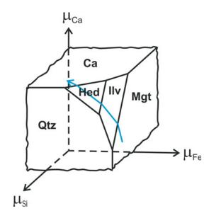
FIG. 12. Diagram of the chemical potentials to account for the zoning sequence magnetite – ilvaite – hedenbergite – marble in the skarns, after Burt (1977) and Rose & Burt (1979).
