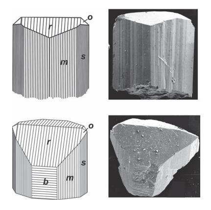
FIG. 6. Morphology of manganilvaite crystals with forms (in the structural setting)  $r\{011\}$ ,  $m\{110\}$ ,  $s\{210\}$ ,  $b\{010\}$  and  $o\{111\}$ . The crystals are presented with their *b* axis toward the reader (for direct comparison with the crystal drawings of ilvaite published already, given in orthorhombic setting with *a* and *b* axes interchanged and c < a < b).
