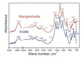
FIG. 5. IR absorption spectra of manganilvaite from Ossikovo and Mn-free ilvaite from Seriphos.
