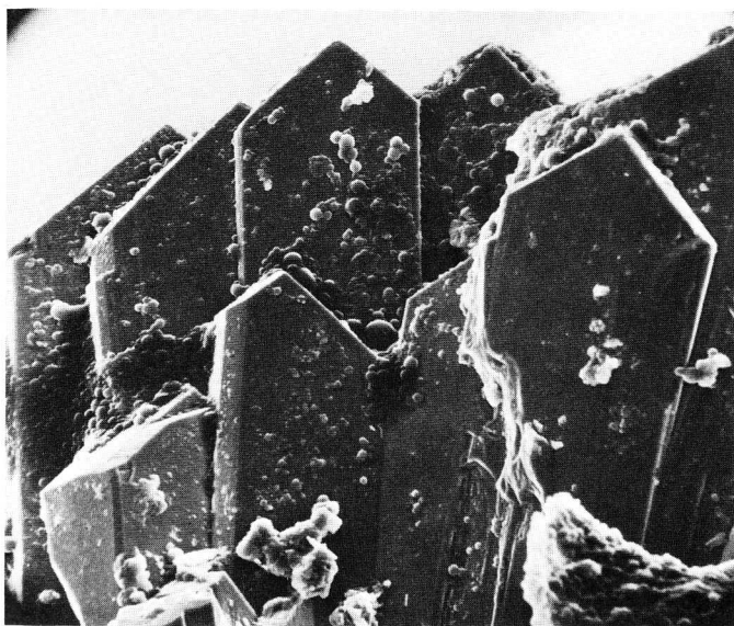
Figure 1. Scanning electron micrograph of a sub-parallel group of bladed nealite crystals from the type specimen. Small spherules on the face of the crystals are glue inadvertently spilled on the crystals during mounting. NMNH 137115 (280x).
