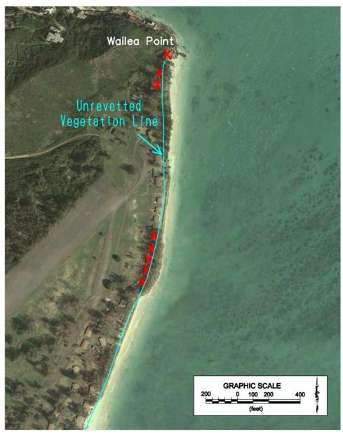
Figure 36 Shoreline response to removed revetments—Bellows AFS (The red Xs mark cottages and other buildings that may be threatened by the shoreline recession)
