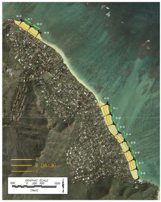
Figure 28 Beach nourishment with structures conceptual design--Lanikai
