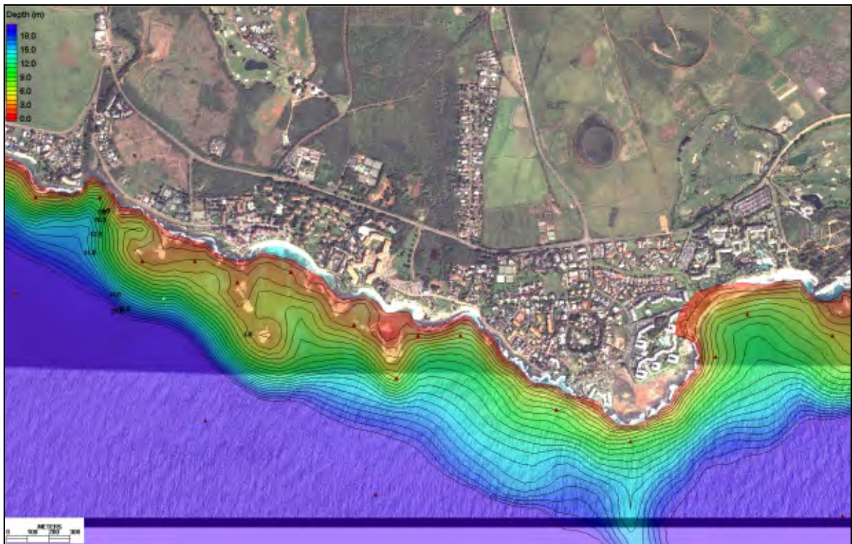
Figure 28. STWAVE Nearshore Grid Adjacent to Poipu Beach in Poipu Region (1m contours shown)
