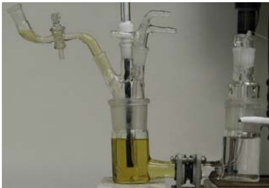
Figure II-5. Electrochemical set up for electrolysis experiments.
