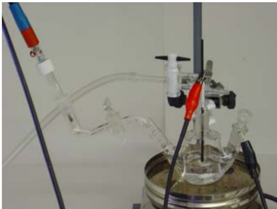
Figure II-1. Electrochemical set up for voltammetric experiments.
