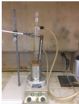
Figure 4. Modified Chapelle test configuration applied to mining residues.
