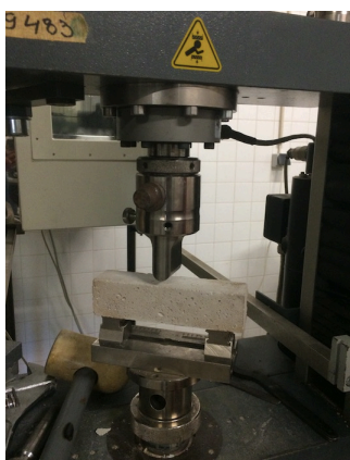
Figure 6. Flexural strength test performed to the mortars produced with mining residues.
