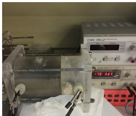
Figure 3. Electrodialytic treatment of mining residues in a 2-compartment reactor.
